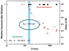
The **critical particle size** below which structural failure does not occur.
