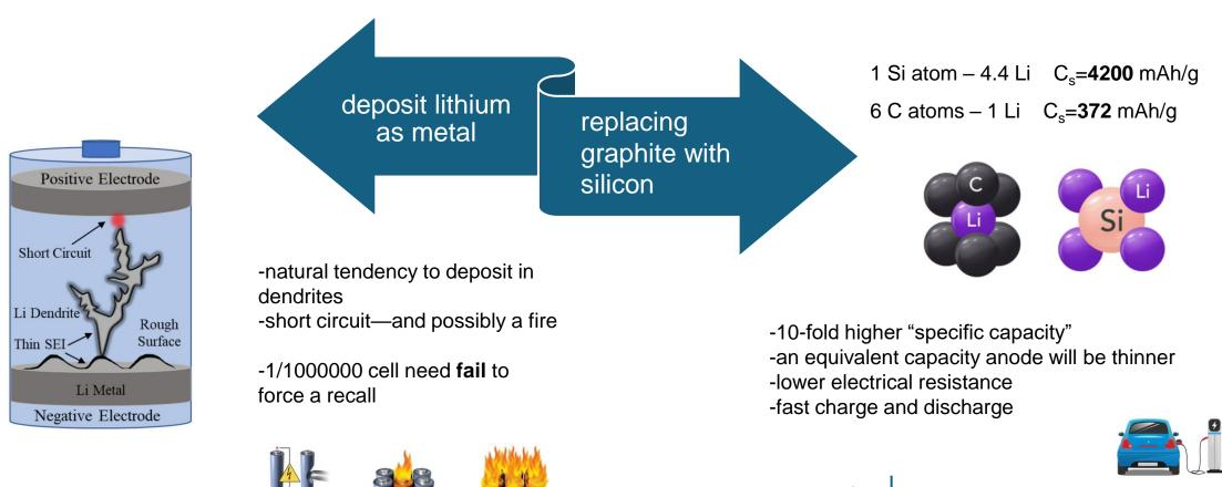
Recharge time Si cell widely regarded as a technology with R<sub>t</sub><10 min
