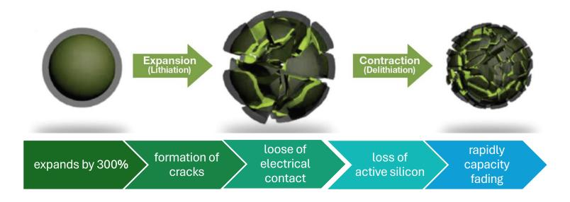
This cycle life limitation in turn limits the amount of silicon that can be added to an EV battery cell.
