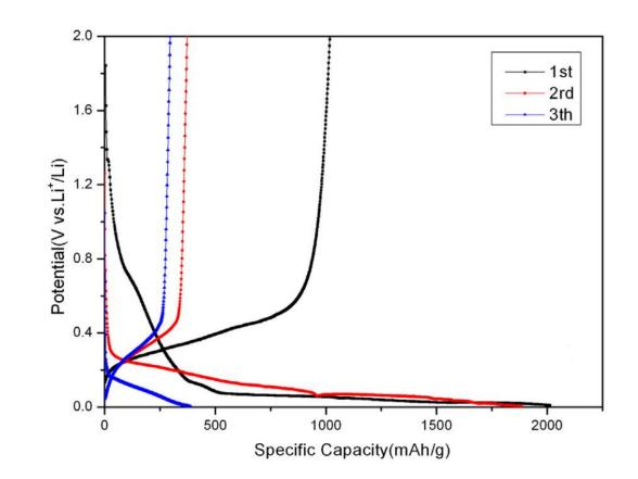
Initial capacity of nano silicon anode are **2013.8 mAh/g** and **1017.0 mAh/g**, respectively, the first columbic efficiency is only **50.5%** and the **specific capacity decays rapidly** in the following two cycles.
